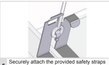
Securely attach the provided safety straps to the installed clips.
