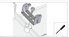
Install the provided clips into the housing, removing existing clips if needed If there are no clips, please confirm housings are SLP Citadel 2 Series.
