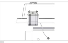
Ground the retrofit kit using the pin nearthe end of the tray in accordance with any current state and federal regulations.
