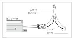
ConnectAC input cables to the incoming AC power connection using the proper connectors in accordance with current state and federal regulations.
