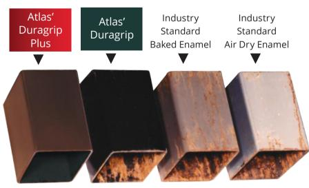
Poles After 1000hrs of Salt Spray Test
