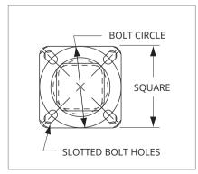
Wide offering of base plates with large range of customization to accommodate existing anchor bolts in retrofit applications.
