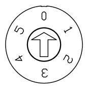
According to the required power, use a flat head screwdriver to rotate the arrow on the switch to adjust the corresponding power.
