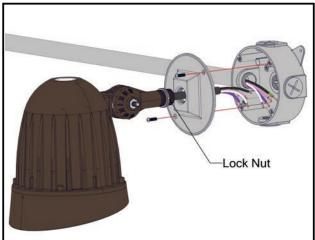
**Step 1:** Feed the power cord into the junction box or conduit. If j-box mounted, insert the threaded portion of the knuckle into the threaded hole of the cover. Secure the fixture with the Lock Nut.
