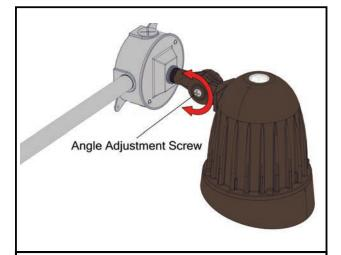
**Step 3:** To aim the fixture, use a screwdriver to loosen the Angle Adjustment Screw. Move the fixture head to the appropriate position and tighten the screw to lock it in position.
