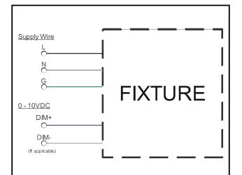
**Step 2:** Make the wiring connections according to the diagram on Page 4. If dimming is not required, make sure the dimming leads are capped.
