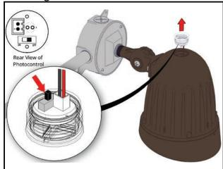
**Step1:** Unscrew the photocontrol and carefully adjust the switch on the back side to enable or disable the photocontrol. Take extreme care not to pull, pinch, or disconnect the photocontrol wires
