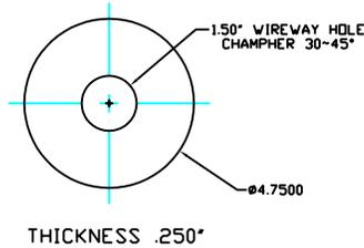
1. PLATE IS WELDED TO 2" ID PIPE ON THE TOP
