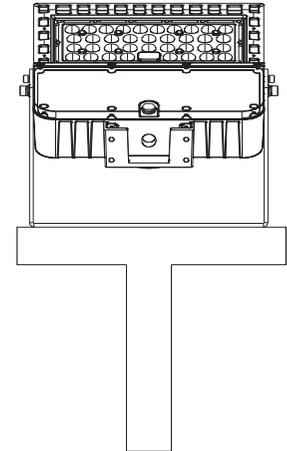
Step 1: Drilled on the pole according to the measurement of hole on the bracket.
