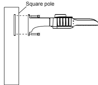
Step 1: Drilled on the pole according to the measurement of hole on the bracket.
