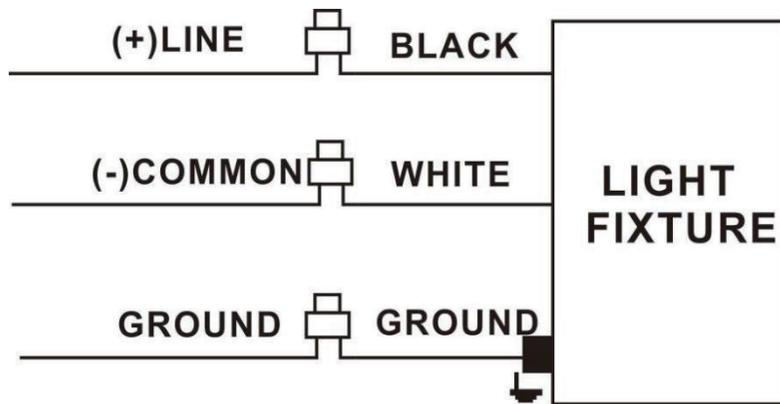
Make the wire connections outside the mounting arm. Refer to the wire diagram for power connections.
