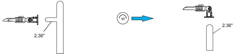
Step 1: Put the fixture with the bracket on the bar which is on the pole.
