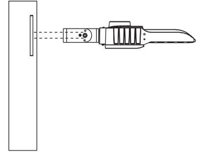
Step 1: Drilled on the wall or pole according to the measurement of hole on the bracket.
