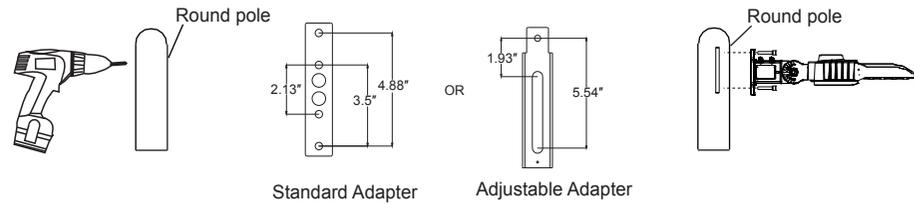
Step 1: Drilled on the pole according to the measurement of hole on the bracket.
