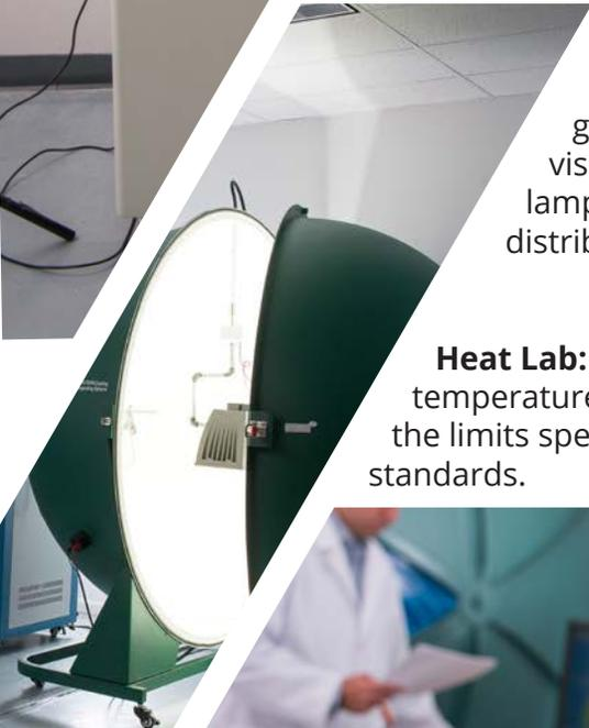
**Integrated Sphere Testing:** The integrating sphere is used to gather fixture output data by measuring the light spectrum that is visible to the human eye. From this data we are able to extrapolate lamp lumens, color temperature, color rendering index, spectral power distribution, voltage, wattage and current.
