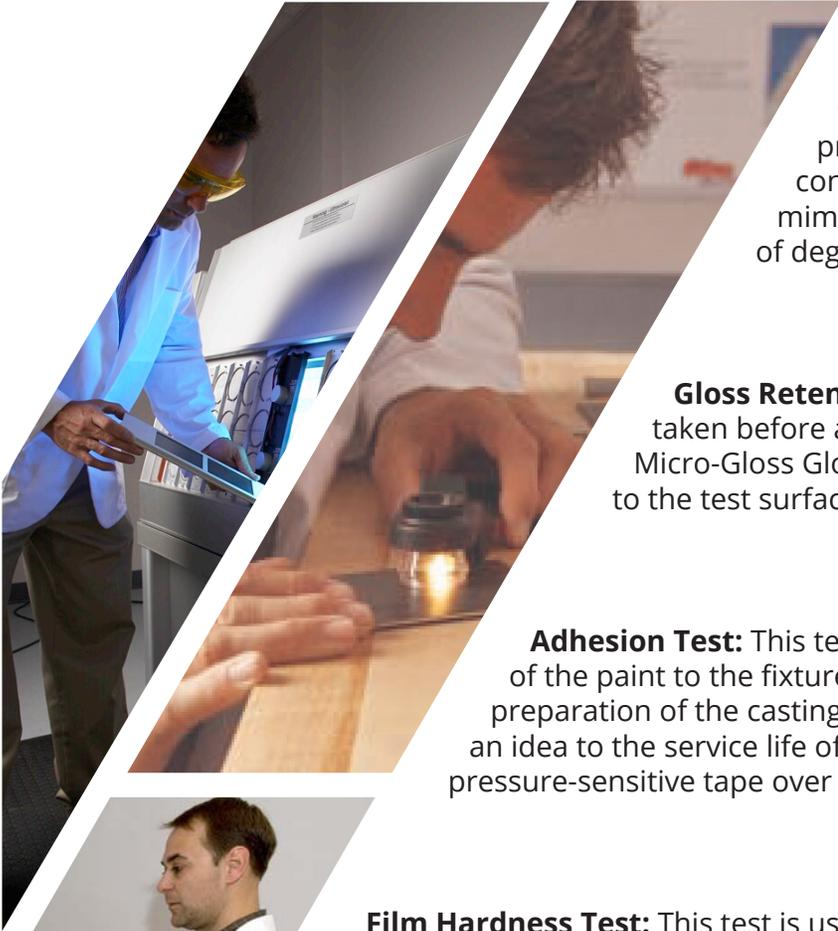
**UV Test:** Each product undergoes a test in a weathering chamber which produces cycles of simulated sunlight, condensation and temperature change to mimic the environment and measure degrees of degradation.
